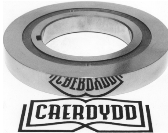
Figure 4: A superfinished steel test disc showing high quality finish achieved.
